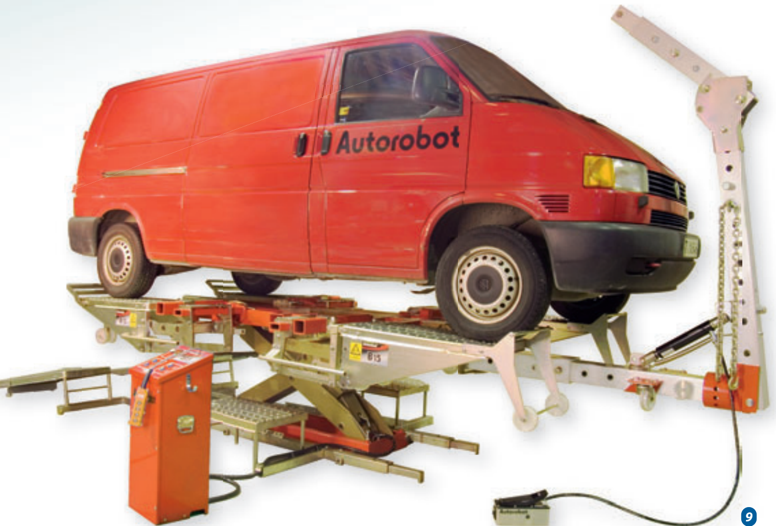
Autorobot B15 is equipped with electric hydraulics controlled from the control desk or remote control panel.
