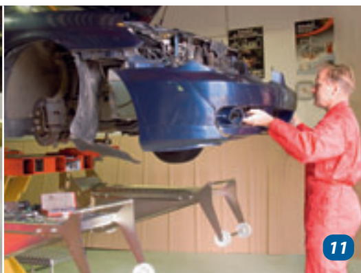
Autorobot B15 performs perfectly in numerous jobs in the body shop. (pictures 10 and 11). Disassembling vehicle parts in good working position.
