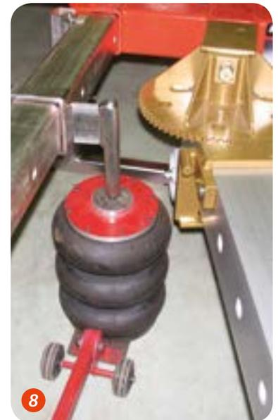
*Pneumatic lift that belongs to B5 basic set makes mounting of a vehicle easy. The collision repair system can easily be lifted to a suitable ergonomic working height with help of the pneumatic lift.*
